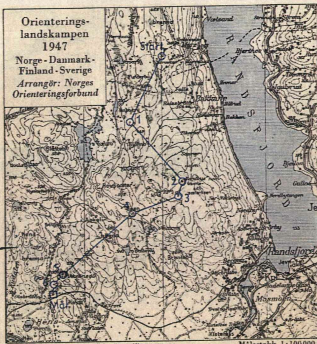
The map from the Nordic Match in 1947. The contour interval is 30 metres. "This means that hills of 25-29 metres might disappear between the contours. As the Swedish, Finnish and Danish participants also did" to cite Skärmen.
